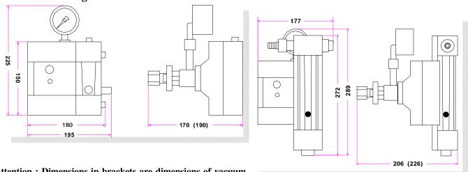
Attention: Dimensions in brackets are dimensions of vacuum regulator equipped with pressure gauge
